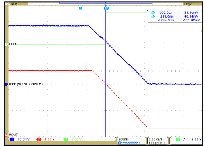
Figure 12. CT430 OCD disabled at 90% of +50 A_{DC} and FLT# is HIGH
