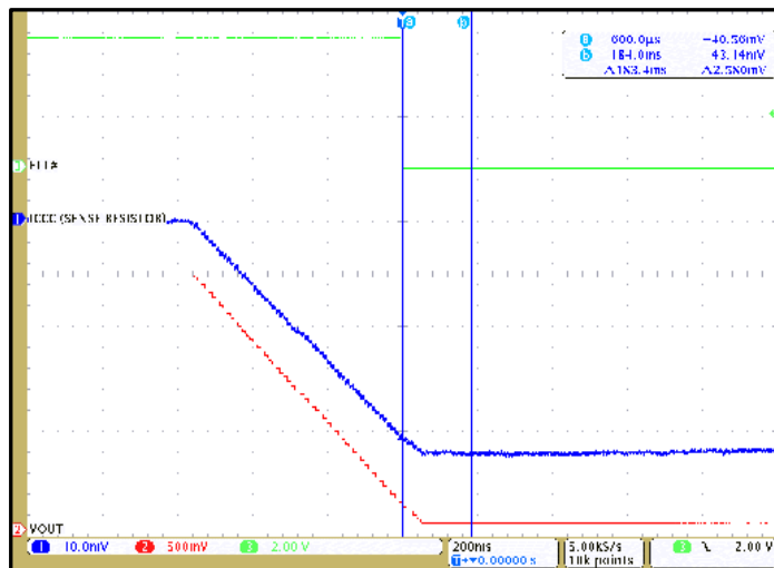
Figure 15. CT430 OCD enabled at -110% of -50 A PK and FLT# is LOW
